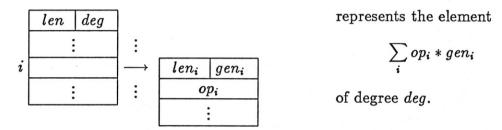
The lists  $Ext^s$  of generators for the resolution in cohomological degree s are examples of lists which need to be able to grow. To keep such lists in a single block without having to recopy them each time an element is added, we use a block whose length field is the full length 2n-1 of the block, while the key field is set to the actual data length of the block. When the block is full, we copy it into a new block with some room to spare for expansion.
