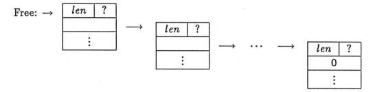
If less than an entire block is being returned, it is taken from the end of the first large enough block. In this way, no pointers in the free list have to be changed.
